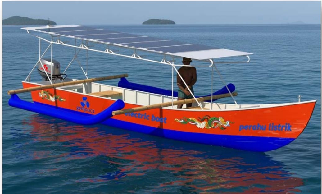
With 3kW Solar panels, four battery packs can be fully recharged in eight hours
